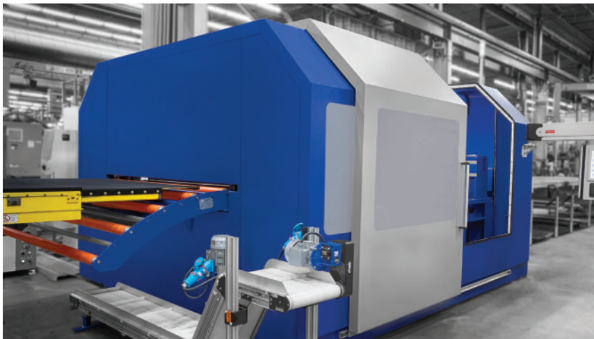
With coil-fed laser blanking, production doesn't need to stop when a line goes down or a die needs maintenance. Another laser line can take the drawing and begin cutting parts. (Right, the laser head.)
